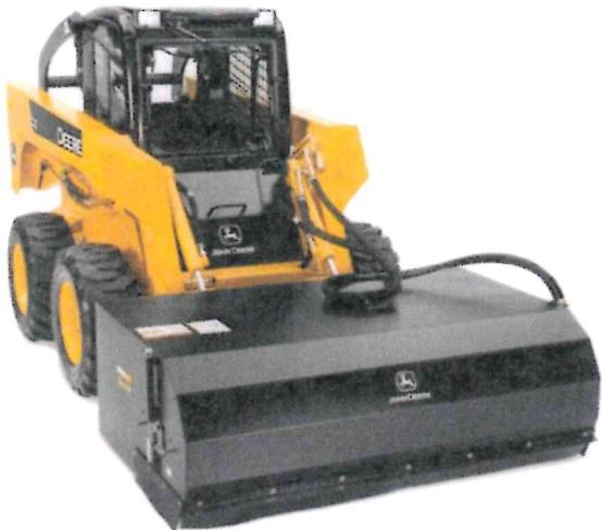
Like all Worksite ProT attachments, these pick-up brooms are optimized to work with John Deere Skid Steers and Compact Track Loaders, 244J Loader, and 110TLB. They're compatible with many competitive models, too.
